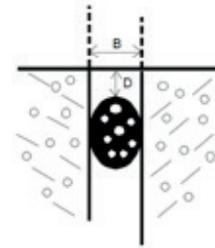
Materials used as backer rods should be weaker than the sealant itself and not obstruct the movement of the sealant, whilst compressing or expanding. Most suitable backer rods are:
